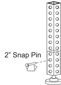
The leg sockets on the stage sections fit 1-3/4" sq. stage legs. Use one of the following only:
